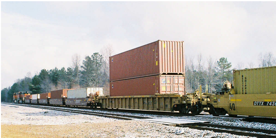
Figure 5.1 Doublestack container wellcar at Myrtle, Mississippi. Photo Credit: James A. Burt.
